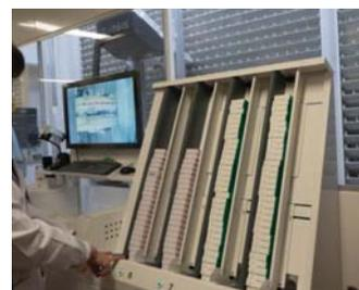
**Picture 4.** Refilling the Rowa Vmax Box Picking Machine
